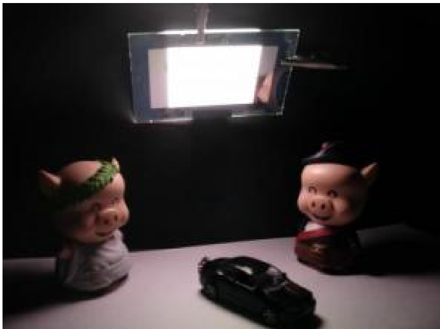
Light produced by a new type of light emitting diode (LED) made from inexpensive, plastic-like organic materials. (Credit: Photo by Ma Dongge)
